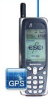
Benefon Esc! This was the first instance of a GPS being integrated into a mobile phone.
